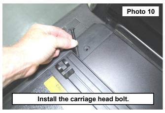
11. After ensuring the carriage bolt is fully seated, thread the supplied knob nut onto the carriage head bolt. Then thread the wing nut onto carriage head bolt and slightly tighten the knob nut to the wing nut. **See Photos 11 and 12.** Note: These nuts will not be tightened until the cover has been adjusted to ensure full latch engagement.
