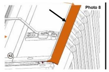
10. Ensure the cover is pushed up to the front of the bed and centered side to side in the aluminum track. Place the supplied carriage head bolt into the front hole of the cover. See Photos 9 and 10.
